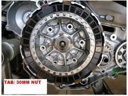
3. Remove clutch plates and inner hub.
