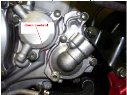
2. Drain coolant (remove radiator cap)
