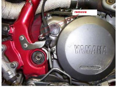
5. Remove rear brake pedal/master cylinder assembly & move back out of way.
